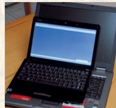
Small is beautiful. A netbook computer, compared to a laptop, requires much less electricity, making it perfect for remote locations where solar power is the only option.
